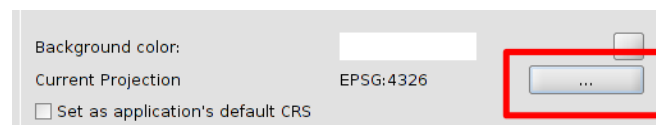
Figure 1. Button where reference system of a View can be changed in gvSIG
