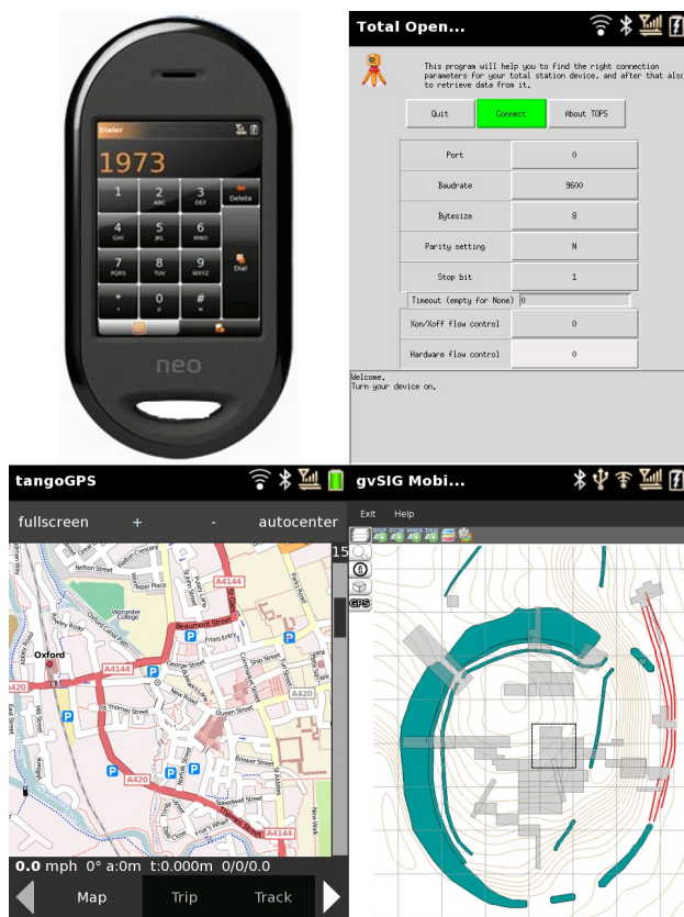
Figure 5: The OpenMoko FreeRunner device and some applications running on it (Total Open Station, tangoGPS and gvSIG Mobile).
