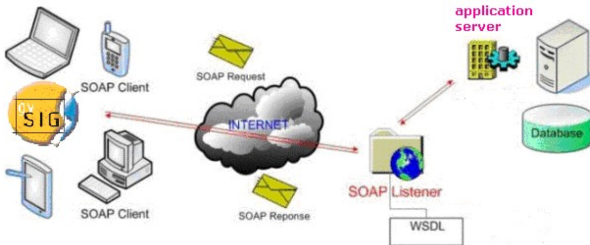
Fig. 1: Communication between Client and new Infrastructure (newGIS)
