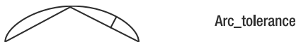
Figure 9-2. The arc tolerance is the maximum distance between the arc and the lines approximating the arc.
