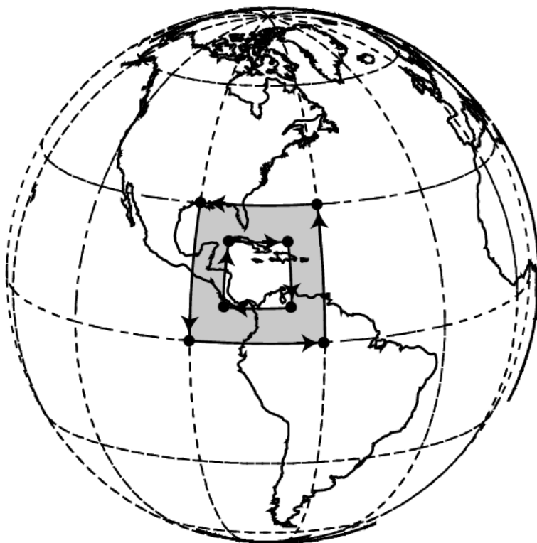
Figure 2-3. Ring orientation of a Polygon containing two rings
