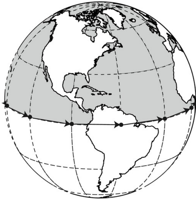
Figure 3-2. The importance of Polygon ring orientation using the geography datatype. Does the Polygon created from the ring shown here contain the Northern Hemisphere, or the Southern Hemisphere?
