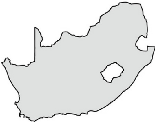
Figure 2-15. A Polygon containing an interior ring, representing South Africa. The interior ring represents the border with Lesotho.
