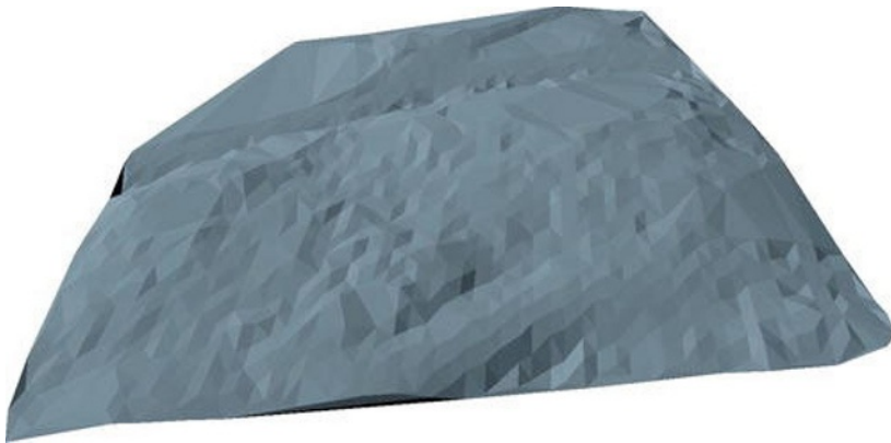
Figure 15-10. A triangulated 3D surface from LIDAR data of Wolf Point viewed in WPF
