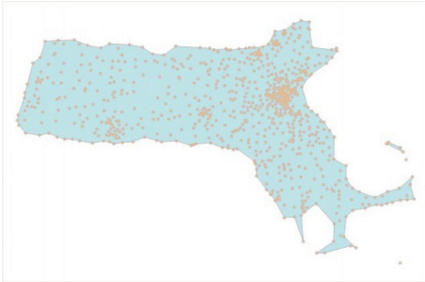
Figure 15-15. An alpha shape created from the firestations in Massachusetts using an alpha value of 11,000
