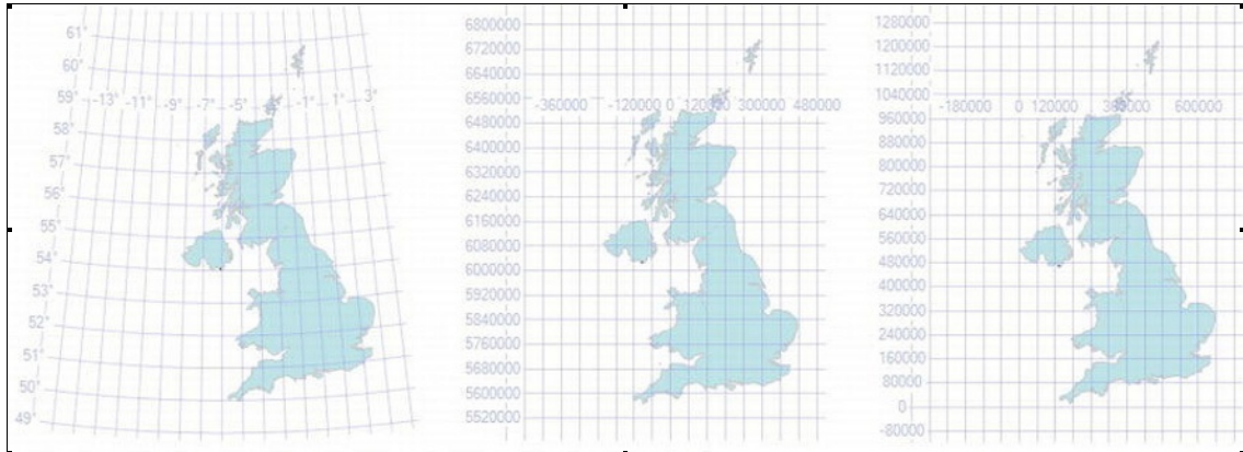
Figure 8-10. Three different projections of Great Britain. From left to right: geographic (EPSG:4326) using Bonne projection, UTM Zone 31N (EPSG:32631), Ordnance Survey National Grid of Great Britain (EPSG:27700)
